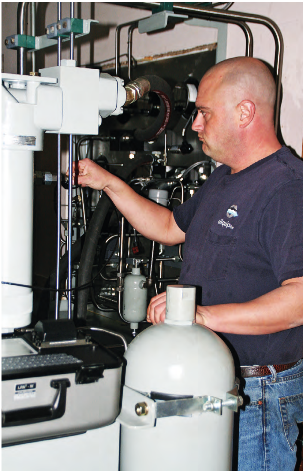
Fig. 1. Service technician uses portable laser particle counter to determine if hydraulic oil is within ISO compliance standards.
