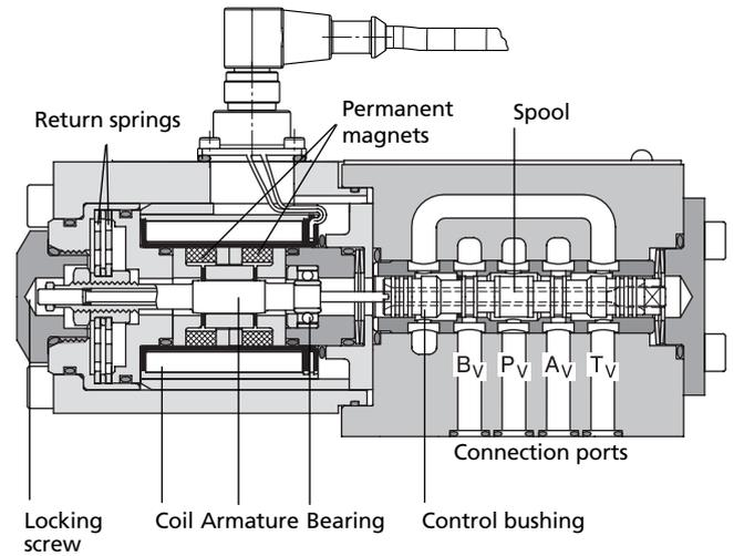
When returning to the center position, the spring force and the drive force act in the same direction. In the center position defined by the centering spring the linear force motor does not consume any current.
