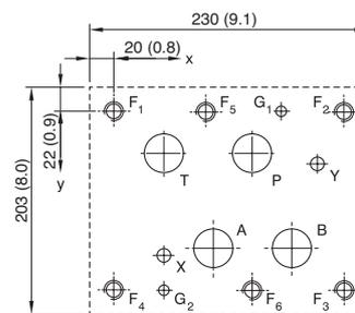
\* Dimension not according to ISO but EN 24340. The position of the mounted safety pin is according to EN. Hole G1 according to ISO is 138.6 mm (5.46 in) and it is drilled in the valve body in line with ISO.
