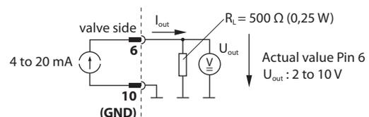
(For signal type "D",  $R_L$  is in the valve electronics)
