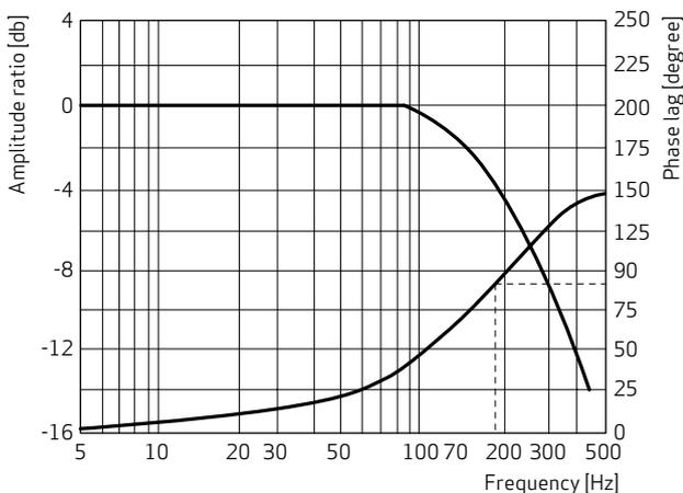
A valve's dynamic response can be easily determined by measuring the frequency at which the phase lag between the input position signal and output position signal reaches 90° (90° phase lag point). The frequency response will vary with input signal amplitude, supply/pilot pressure, and fluid temperature. Therefore, comparisons must use consistent data.
