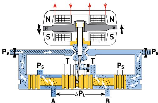
Valve responding to change in electrical input
