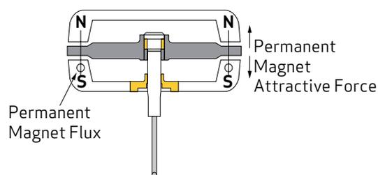
The charged permanent magnets polarize the pole pieces.
