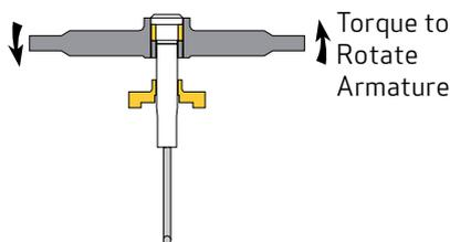
The basic principle is to create a torque that rotates the armature around its fixed point.
