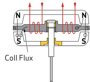
A DC current applied to the coils causes an increased force in diagonally opposite air gaps. The magnitude of the force is proportional to the current. The direction of the force depends on the direction of the current.
