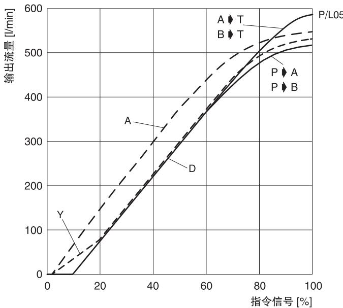
$100 \text{ l/min} = 26.4 \text{ gpm}$
